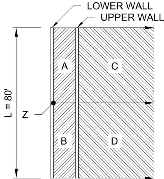
Figure 2: Plan View of Tiered Retaining Wall.
