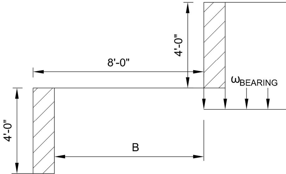
Figure 1: Section View of Tiered Retaining Wall System
